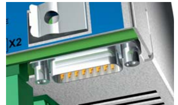
Encoder interfaces for 2 systems: HTL incremental encoder ("24V" for MGS system motors) TTL incremental encoder (RS422, "5V")
